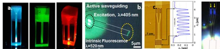
**Figure 1.** **a.** Multicolor visible tri-phenylalanine (FFF)-nanodots; **b.** Active waveguiding in FFF-peptide tape; **c.** Peptide integrated chip: FFF -based 1x2-power Y-optical splitter with grating couplers at all three ports.
